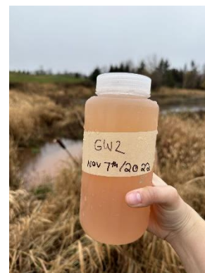
Total Suspended Solids Sample (2022)
