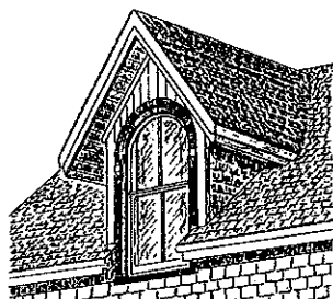
Dormer Window on roof
